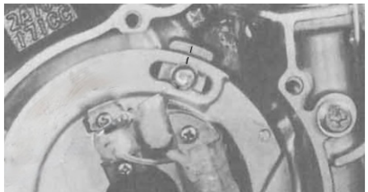
Set up marks used by the factory and described in the shop manual
