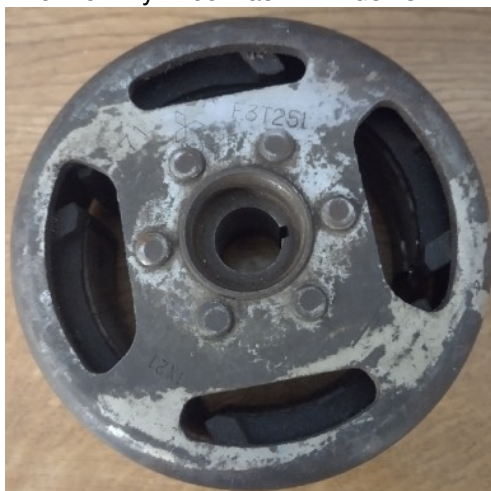
F3T251 Flywheel has 4 'windows'
