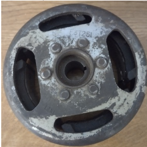
F3T251 Flywheel has 4 'windows'
