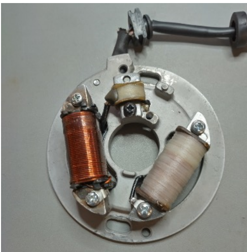
Single source coil, mounted on the right of the pick-up.
